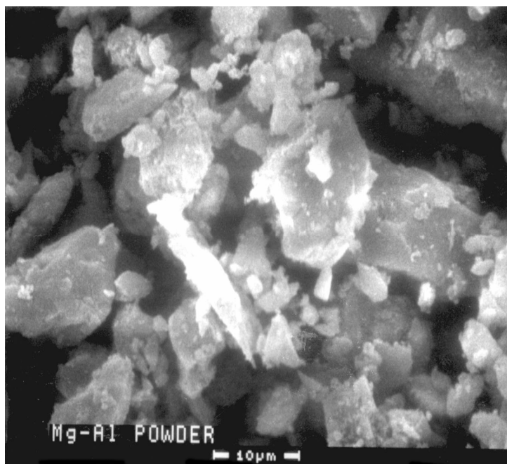
Photo 5. Electron microscope picture of milled Mg/Al alloy used in this study.
