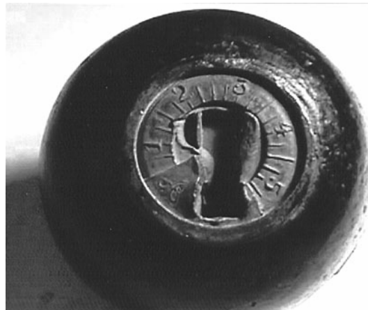
Figure 3. A photo of a Bormann fuse in place on a 6-pounder cannon ball.
