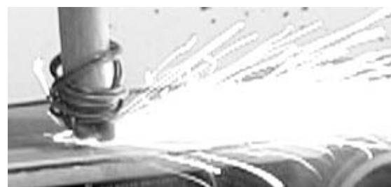
Figure 11. Photographs of the friction test setup as modified for e-matches. There is a time lapse of 1/60 th second between images.
